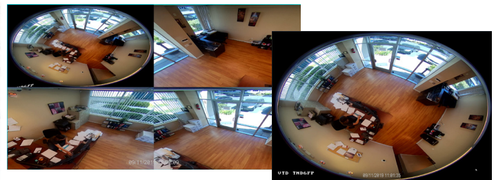
Fish Eye De-Warping: Multiple Views include 360° Overview, Double 180° Panorama View, Quad View, Overview + 3 Views, and Single View
