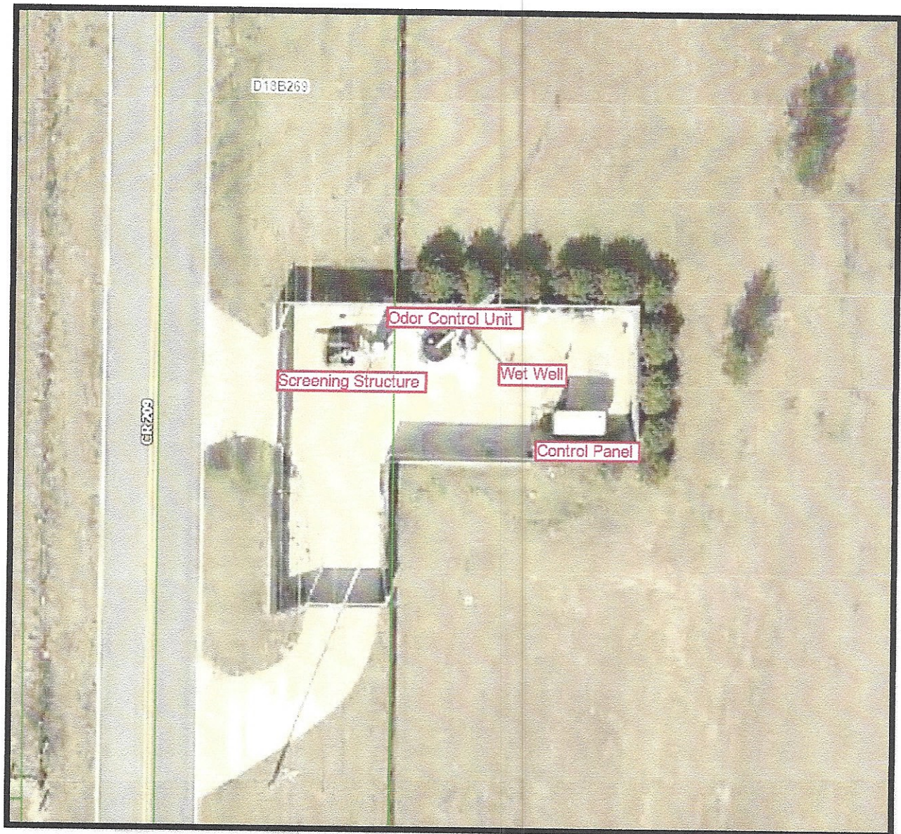
FIGURE 2 – COUNTY ROAD 209 LIFT STATION EXISTING EQUIPMENT
