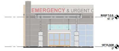
A2 WEST ELEVATION - ENTRANCE CANOPY SCALE: 1/8" = 1'-0"
