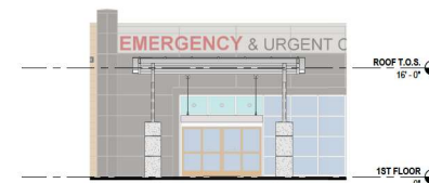
A2 WEST ELEVATION - ENTRANCE CANOPY SCALE: 1/8" = 1'-0"
